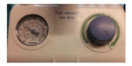
Ensure that the indicator on the vacuum knob is aligned with the green arrow.
