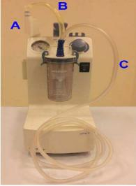
3. Switch the vacuum pump on and Cover the tube with your finger. The vacuum gauge should read at least 575 mmHg. Remove your finger. The vacuum gauge should drop drastically (to zero or close to zero). If the vacuum unit complies with the above behavior, the vacuum unit is functioning properly. If the vacuum fails to reach 575 mmHg or fails to drop to close to zero, the vacuum unit should not be used. Contact customer support.
