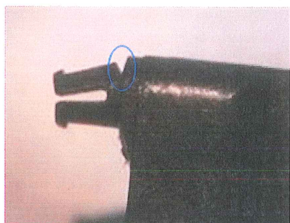
Half of the pin damaged
