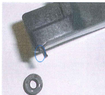
Half of the pin broke off
