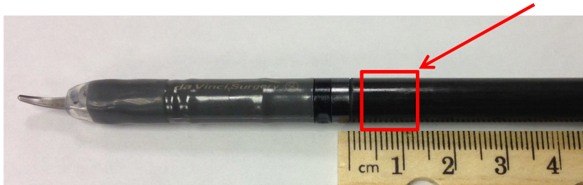
Figure 1: Location of micro-cracks
