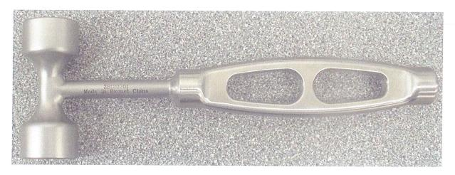
Biomet UK Ltd has initiated this action following an investigation that indicated that excessive use of the instrument could result in cracking on the weld between the head and the handle. This could lead to part of the head becoming detached from the handle.
