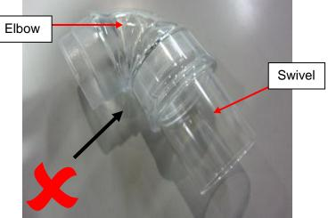
Figure 4: Incorrectly assembled vented elbow with missing NRV valve
