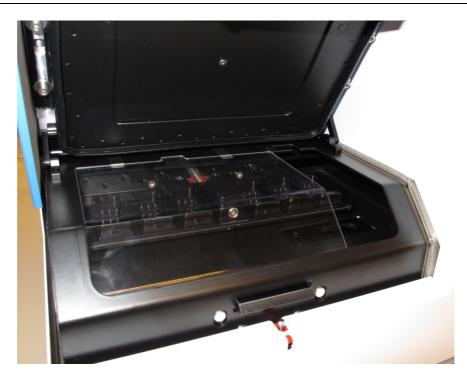
EmbryoScope time-lapse incubator with open load door and transparent plastic cover plate in correct position
