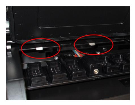
EmbryoScope time-lapse incubator load area with cover plate removed and metal clips in correct position
