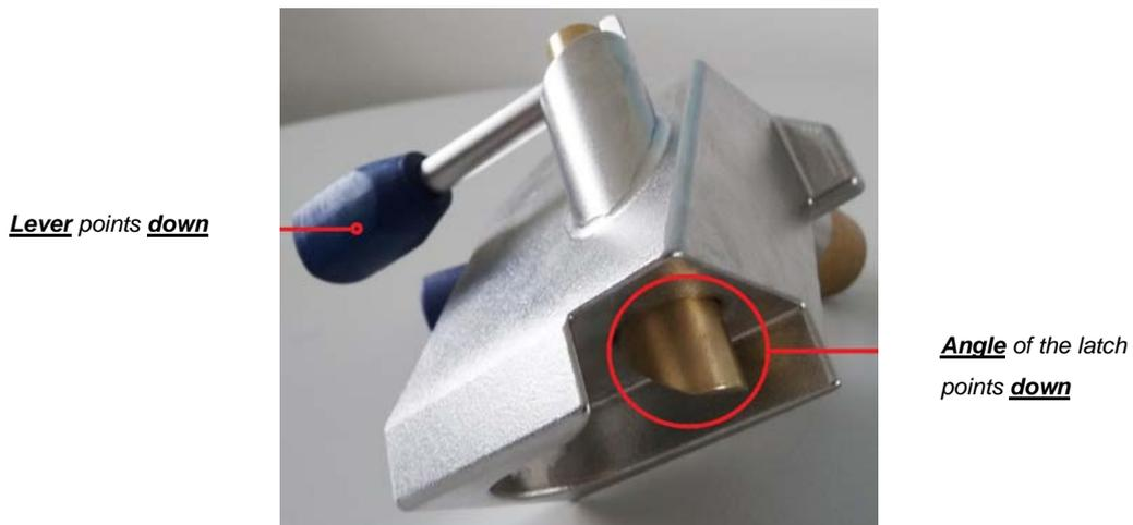
Figure 2: **Incorrectly** mounted latch
