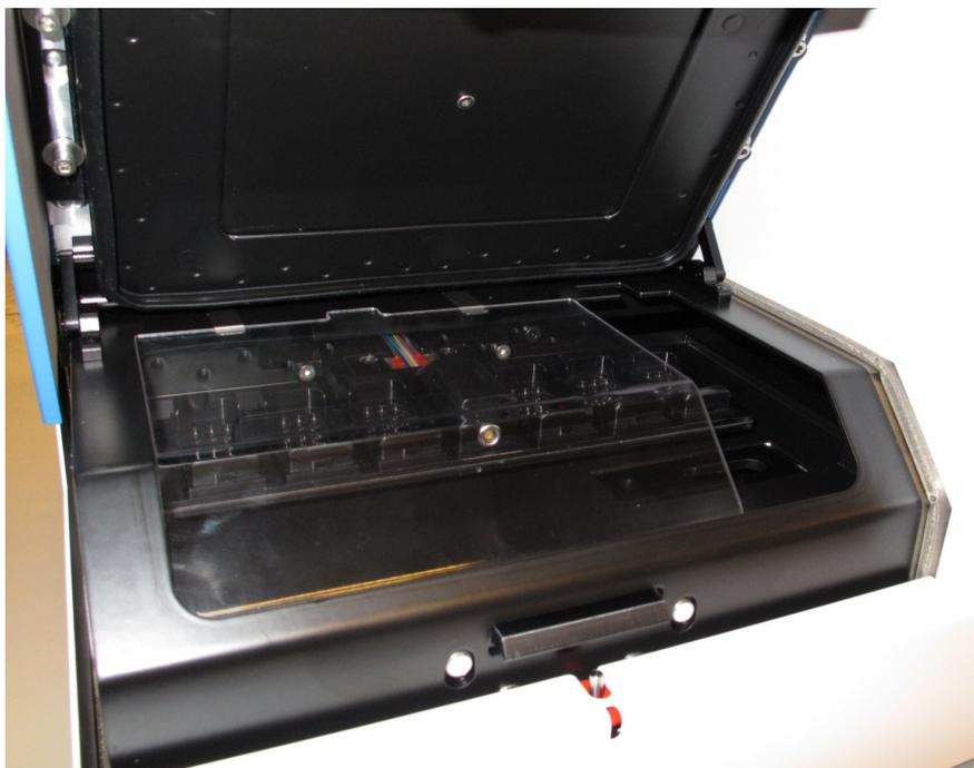
EmbryoScope time-lapse incubator with open load door and transparent plastic cover plate in correct position
