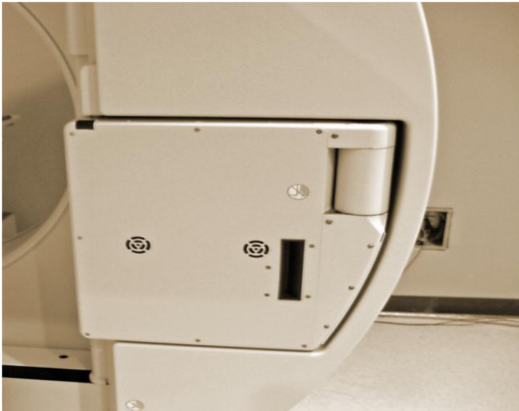
Figur 2 - indfoldet fladpaneldetektor (FPD)
