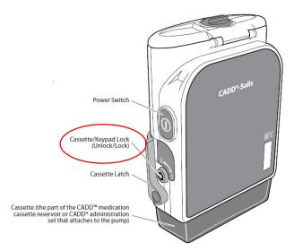
If the user is unable to fully engage the Cassette/ Keypad Lock, then Model 2111 and 2112, and Model 2120 in PCA mode, the keypad will be locked and the pump cannot be started. This could cause a delay in the start of an infusion or interruption in therapy if changing a disposable, while an alternative pump is obtained. A delay or interruption of delivery of pain medication may result in escalation of patient pain based on the underlying condition of the patient. Based on Page 1 of 3
