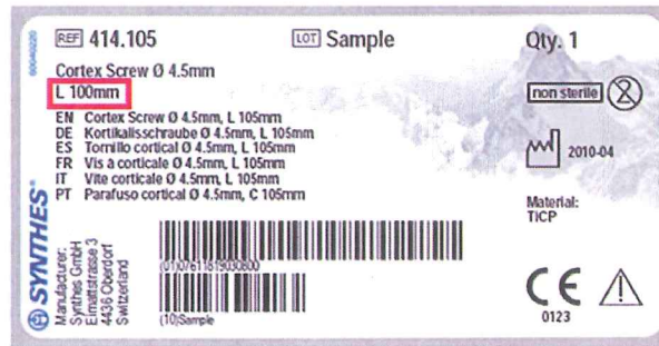
Figure 1 – Incorrect Label for Part 414.105
