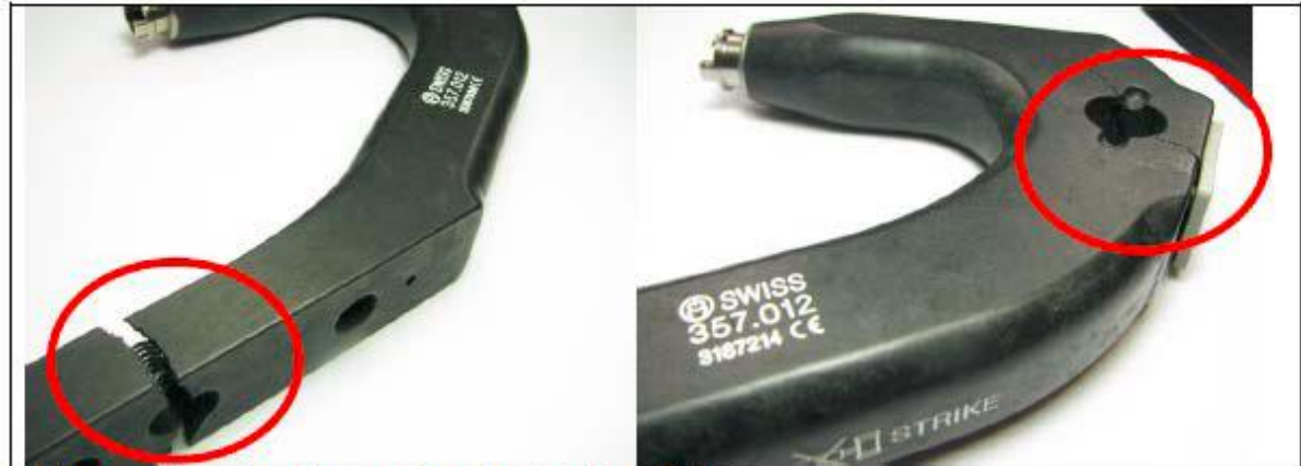
Pictures: Example of broken Insertion Handles 357.012
