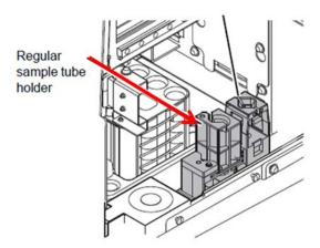
If the described host communication error appeared during XN-550 sampler analysis, check the sample tube holder as indicated in the image and remove the sample tube, if present, before accepting the error message and restarting of the sampler.
