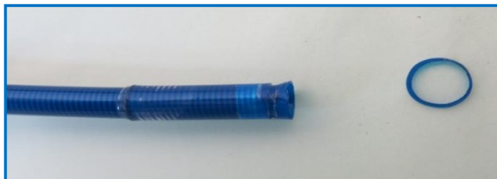
Figure 1c: Small section of the tapered end of the blue sheath detached from the slider collar following retraction of device
