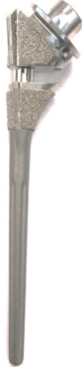
Stem & Body Engagement with Incorrect Screw Assembly
