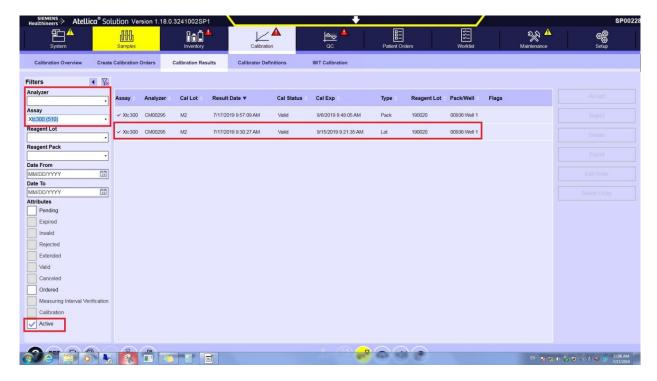
Figure 1. Calibration Results Screen
