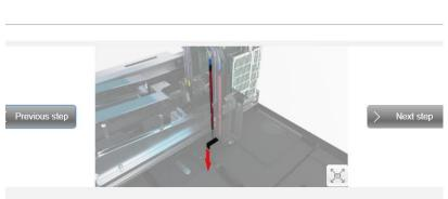
While ensuring that the probes are not bent, carefully remove the drip trays in a downward motion beginning with R1.
