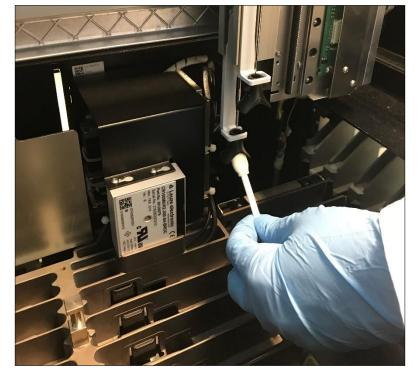
7. Moisten the cleaning swab with disinfectant, and clean the inside of the tube holder.
