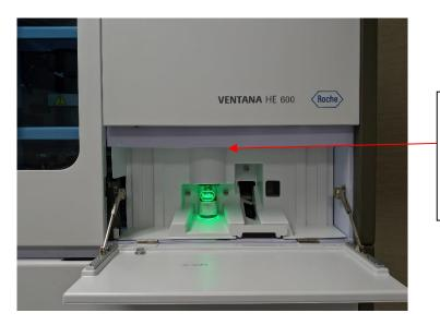
If droplets are observed on the top part of the coverslip module, stop instrument operation, unplug instrument, and contact your local Roche Service organization
