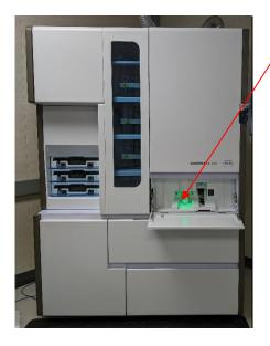
Following the removal of the Coverslipper Module LED PCBA cable, the green light on the coverslipper activator shield will not operate as expected. The green light will be off.
