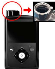
Image: Location of the retainer ring on the MiniMed™ 600 series insulin pump
