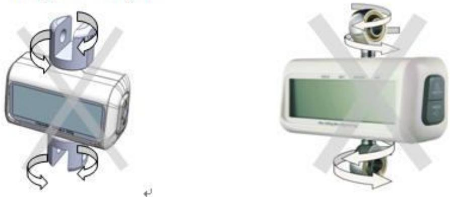
♦ We do not recommend to build in a scale into the construction of any lift or Hoist that hanger bar do not swivel 360 degrees. ♦
