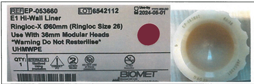
EP-053660 Ringloc-X E1 HiWall Lot number 6542112 contains EP-063660 (Ringlox-X E1 10 Degree ) Lot J6504901
