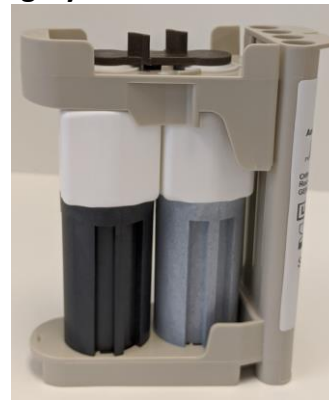
INCORRECT CONFIGURATION grey bottle near wells
