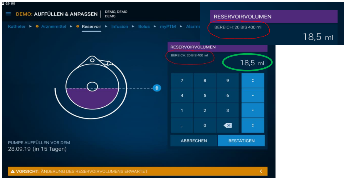
Figure 1: Incorrect values displayed for the allowed range of the reservoir volume (200 – 400 ml): Data entered by HCP is correct (18.5 ml)
