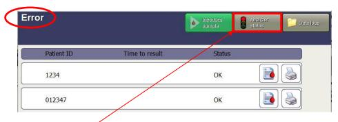
Touch *Analyzer status* to show the condition that caused the analyzer to enter the error state (reset time) and the corresponding message (3264):
