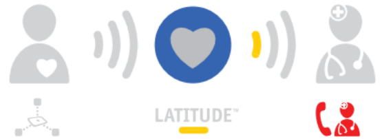
Figure 3. Top : If data transmission is unsuccessful connecting to the LATITUDE System, the Communicator will display one yellow sending wave. Bottom : If a CIED alert condition is not transmitted, the Communicator will display a Red Call Doctor icon.
