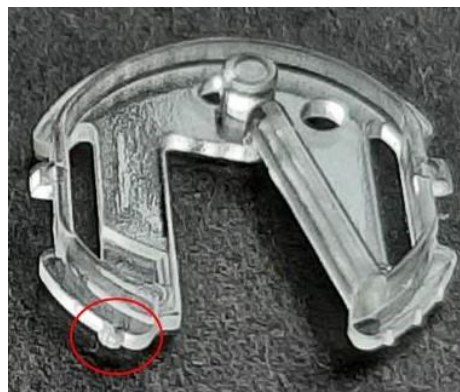
Excess flash (red circle)
