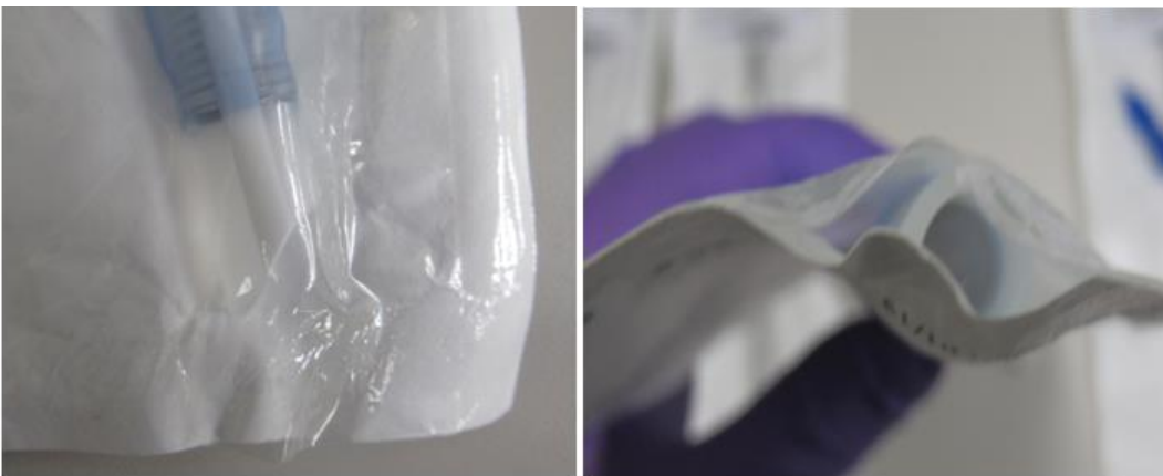
Figure 1. Photo of broken seal.
