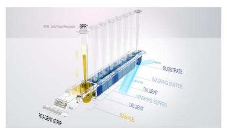
When you are performing a test, if the RFU is higher than the acceptable limit defined during the product development, there is an error message displayed by the system: "Substrate Error". The test is stopped and this alarm prevents the system to provide any result .
