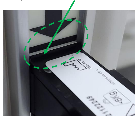
Fig 4 Correct installation (full contact with no gap) of the dovetail mount with the dovetail rail
