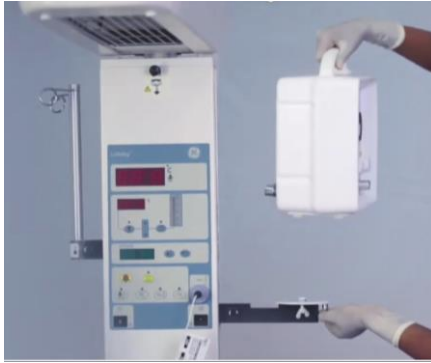
Fig 2. Disconnect and remove Lullaby™ Resus Plus/Prime from the dovetail mount
