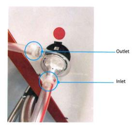
Figure 1: connections of the pump head
