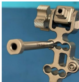
Figure 1: Pin sleeve unable to fit the Infinity™ Alignment Frame Distal Assembly
