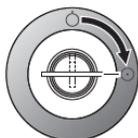
When the key switch is turned on, the exposure condition panel lights up.
