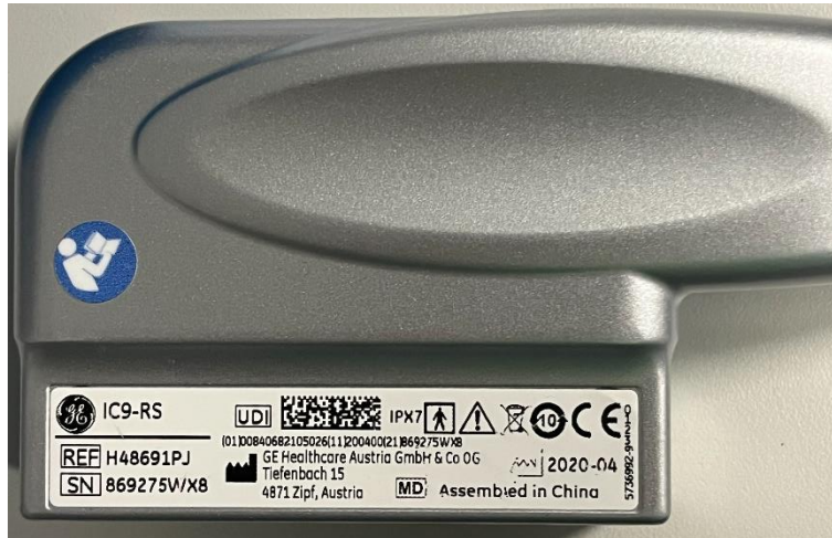
Figure 4. Rating plate example – displaying probe type (IC9-RS) and serial number (SN).
