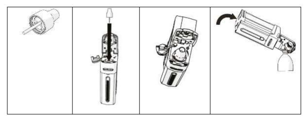
Empty the vaporizer by pouring any remaining agent into a suitable container, which should then be sealed.
