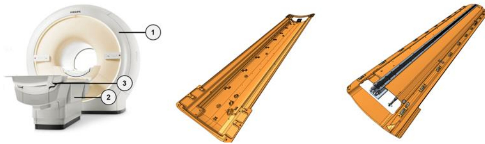
Figure 2. MR System (left image: 1) MR Magnet; 2) Patient Support; 3) IRF Carrier) and IRF carrier (middle and right image).
