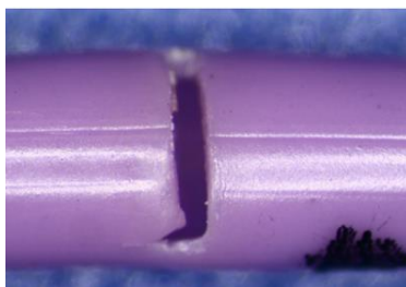
Figure 1: Example of transverse/circumferential crack in the catheter body
