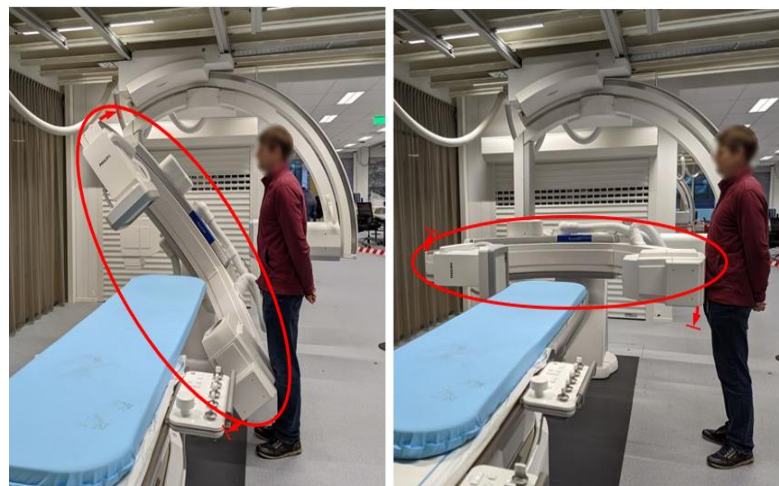
Figure 3: Erratic movements of C-arm (red circle) due to broken propeller motor clamping bolt.
