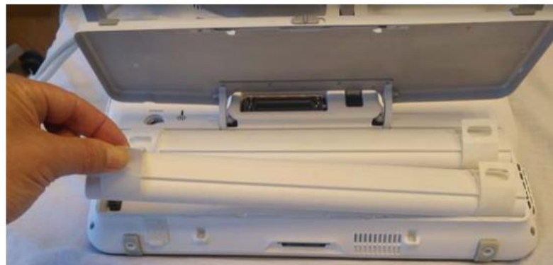
Figure 3-6. Replacing a battery
