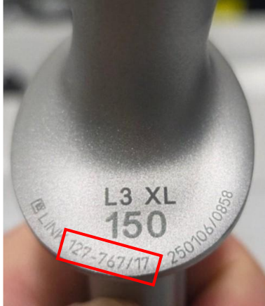
Figure 1: The device laser markings of the affected SPII Hip Stem 127-767/26 show the incorrect Article Ref and CCD-Angle.
