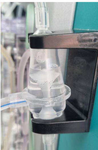
Fig 2: Secure deaeration chamber in holder
