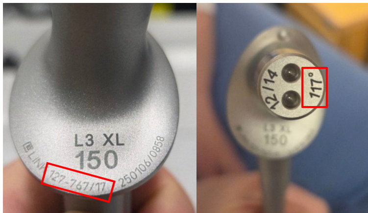
Figure 1: The device laser markings of the affected SPII Hip Stem 127-767/26 show the incorrect Article Ref and CCD-Angle.
