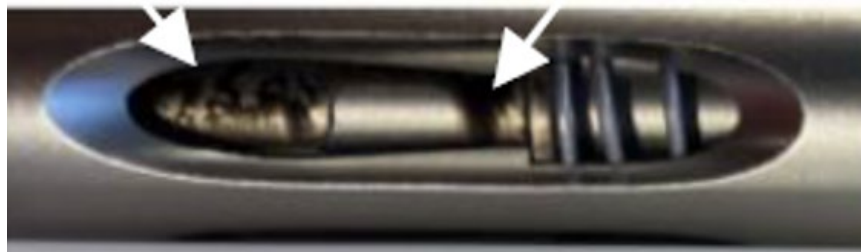
Figure 1: Heterogeneous coating of the Pin Chuck
