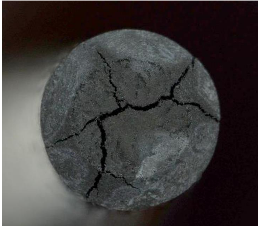
Figure 1: Hoffmann® II Carbon Connecting Rod End with cracking
