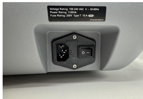
New power entry module
