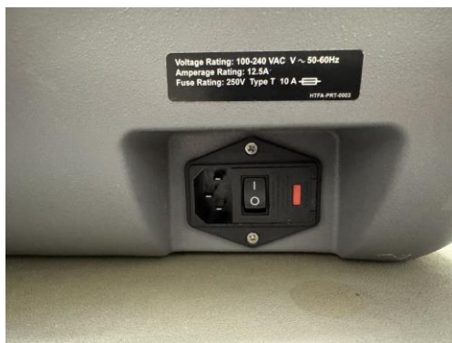
At-risk power entry module (fused cord needed)
