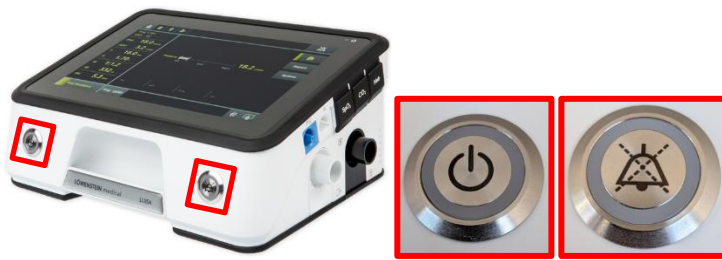
Fig. 1: Press the Power and Alarm keys (outlined in red in this figure) simultaneously for around 10 seconds to force a device reset. After about 10 seconds, the screen will turn black, and the device restarts.
