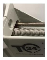
Figure 1: Lead Screw & white plastic debris
