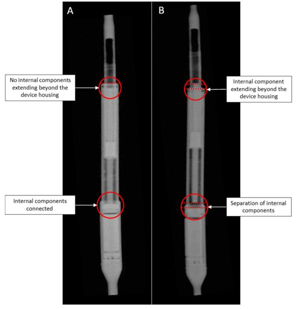
**Figure 1**: Representative X-ray images of a device with an intact locking pin (A) and a device manufactured prior to March 26, 2015 with a fractured locking pin (B). Visual Identifiers of a fractured locking pin can include separation of internal components and the extension of an internal component beyond the device housing.
