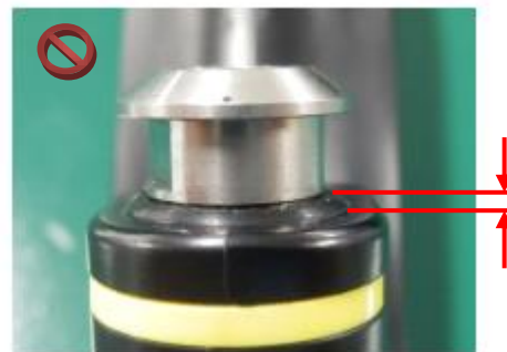
Picture 03: The rubber part lifted
